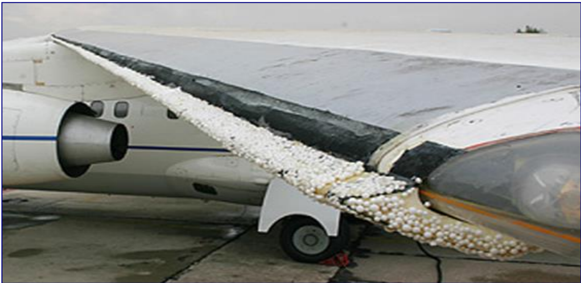
Fig. 4.16. Flight Tests with Ice Simulators
