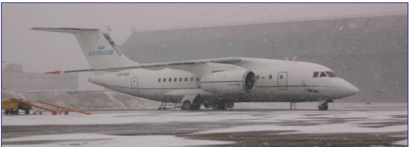
Fig 4.14. Aircraft Test Under Natural Icing Condition at a Temperature of 20° below zero (Arkhangelsk-Naryan-Mar)
