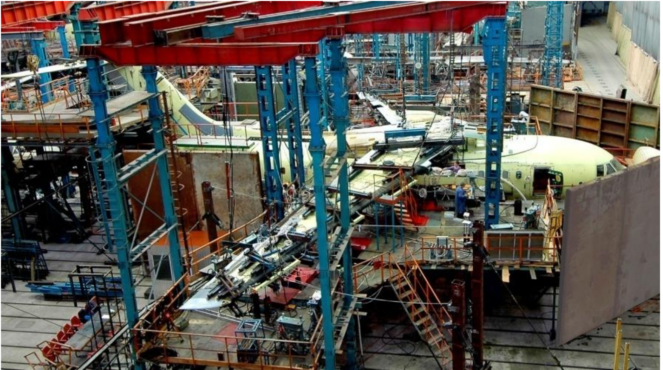
Fig. 3.34. Stand for Airframe Static Tests and Proving Its Lifetime
