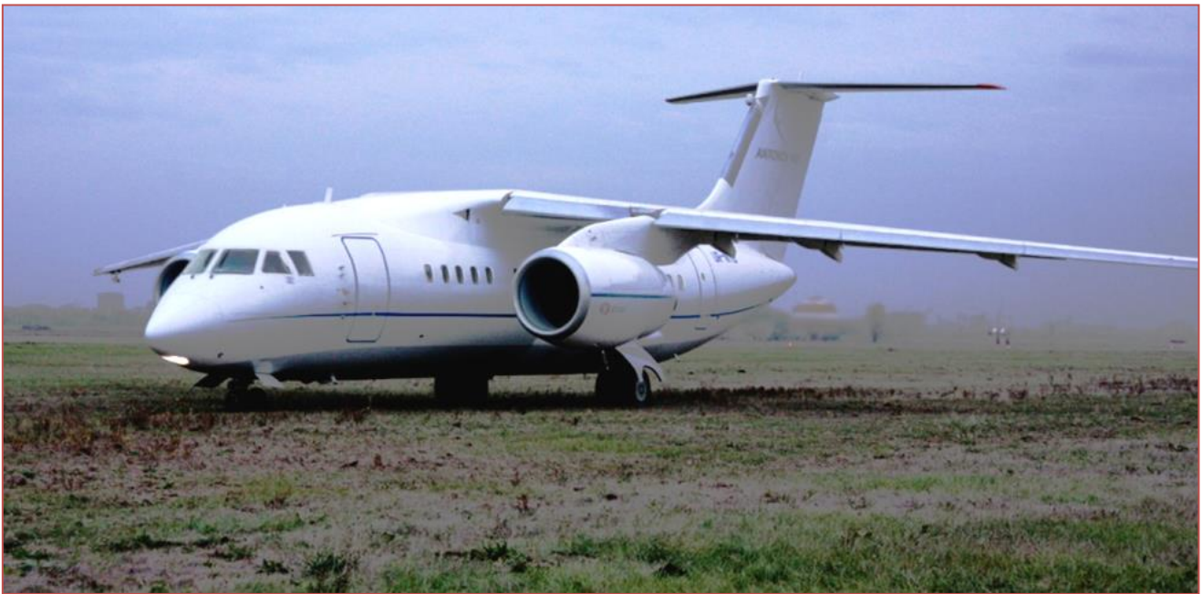
Fig. 4.12. Tests at Unpaved Runway
