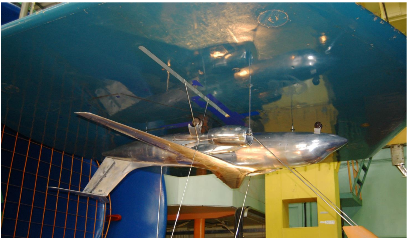
Fig. 3.9. An-148 Aircraft Model Close to Screen in AT-1 Wind Tunnel
