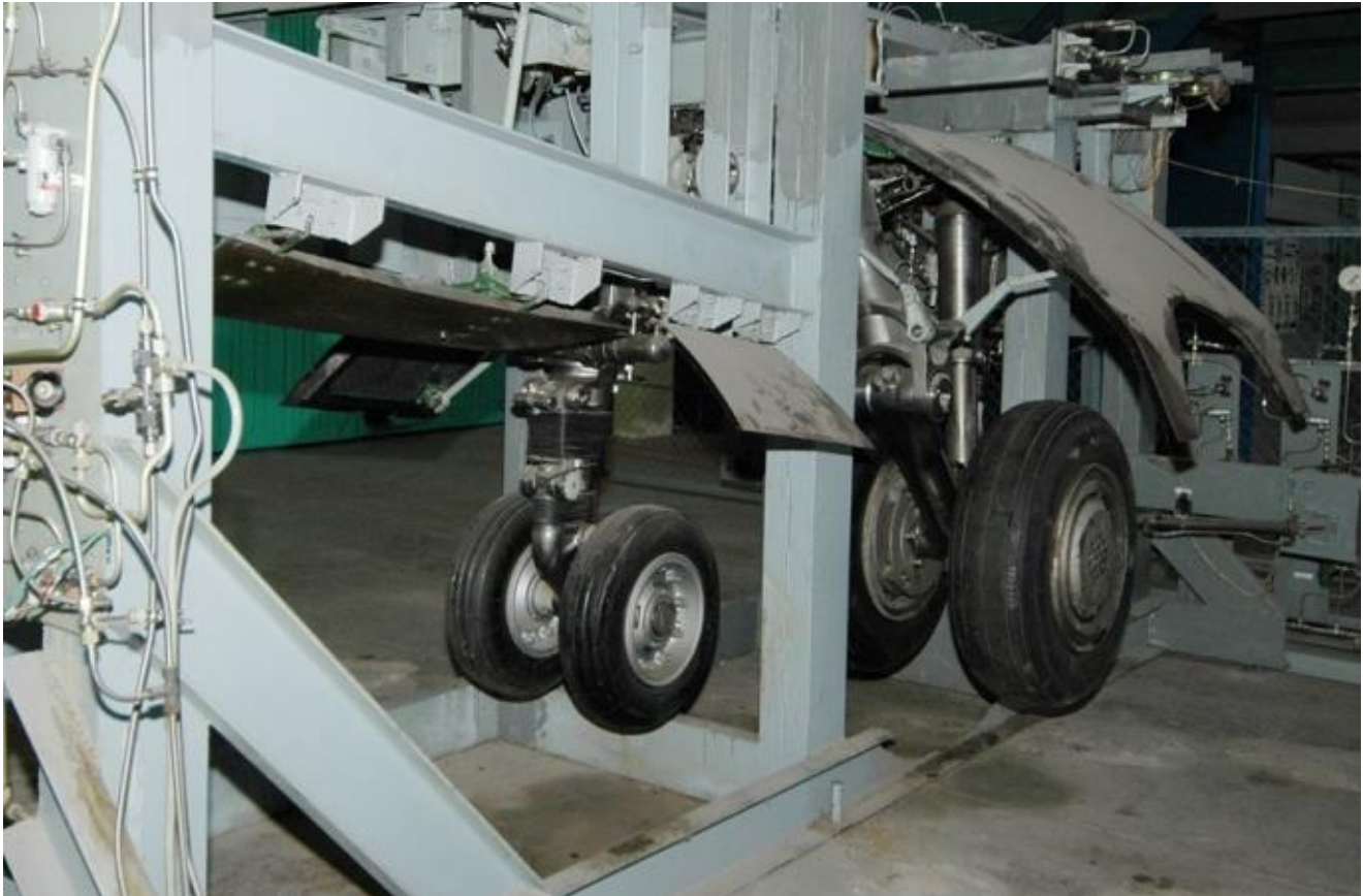
Fig. 4.13. Aircraft Landing Gear Operation Check Test
