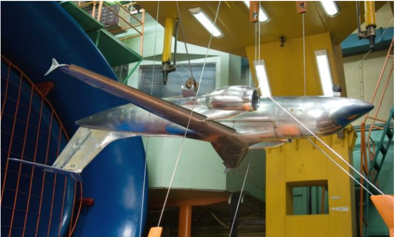
Fig. 3.8. An-158 Aircraft Model fitted with High-lift Devices in AT-1 Wind Tunnel
