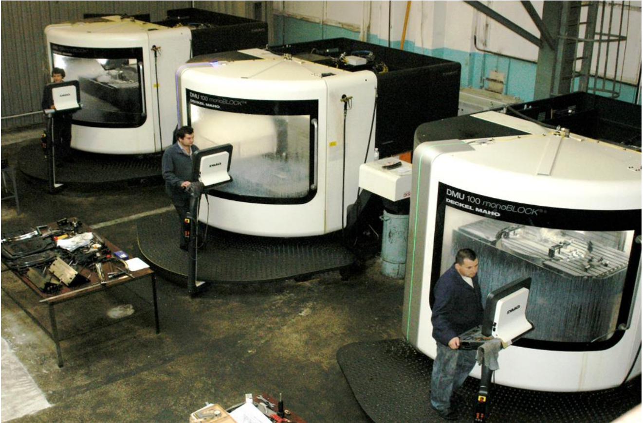
Fig. 4.4. 5-Coordinate Cutting Machine Section
