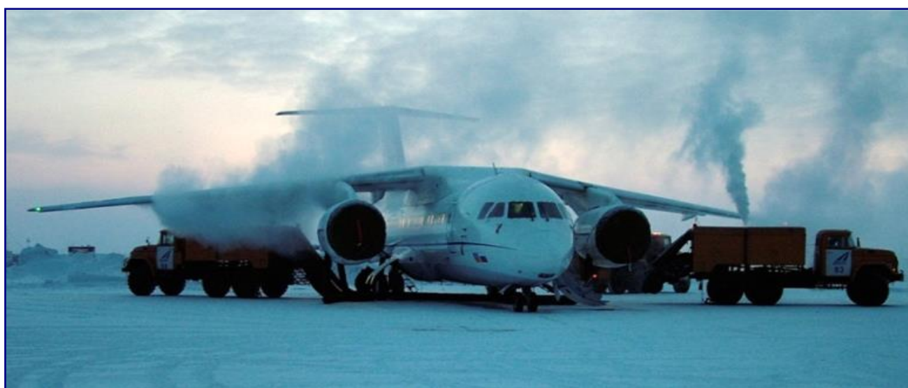
Fig. 4.10. Tests under extreme low temperatures (at minus 55°C), Yakutsk, Nerungri (Russia)
