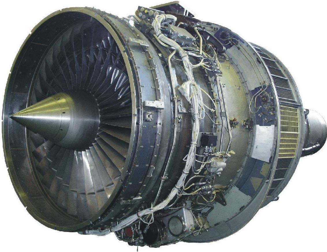
Fig. 2.32. High Bypass Ratio Д-436-148 (D-436-148) Engine
