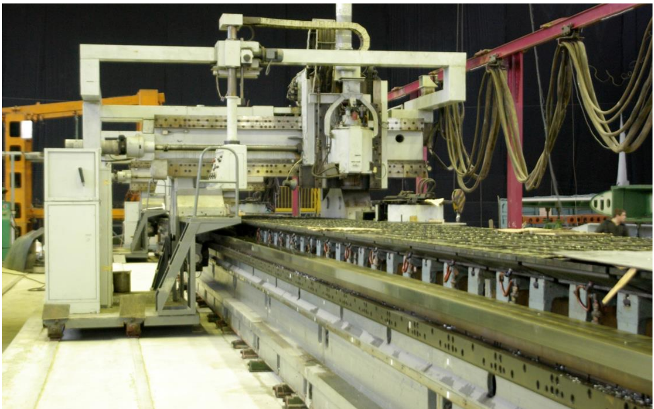
Fig. 4.5. NC Cutting Machine for Fabrication of Long Wing Parts
