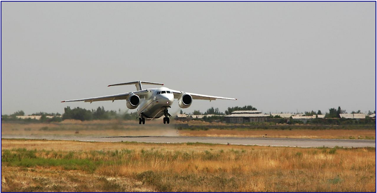
Fig. 4.11. Tests at high temperatures (up to plus 45°C) and under highland conditions (airfields height up to 4100 m. Goumri (Armenia), Karshi (Uzbekistan), Iran, La-Paz (Bolivia)
