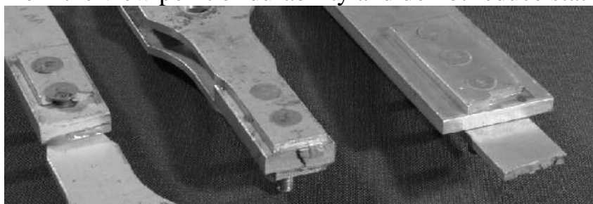
Fig. 8.6. Specimens of bolted joints with local interference
